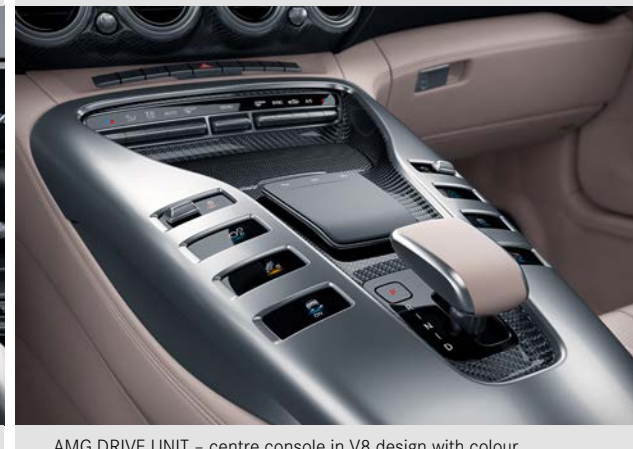
AMG DRIVE UNIT - centre console in V8 design with colour display buttons
