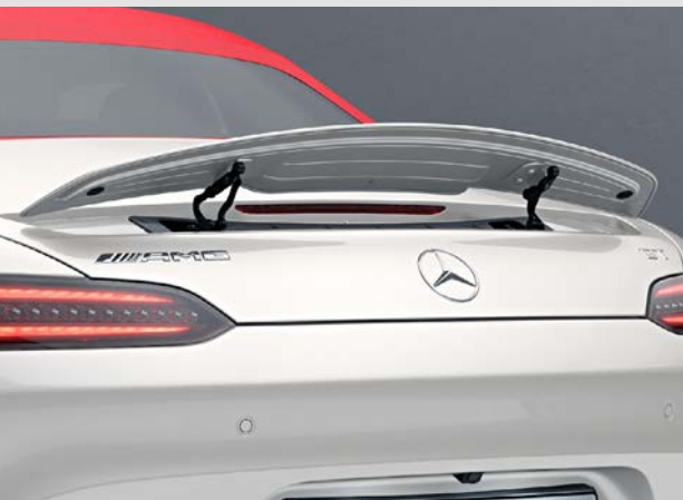
Rear aerofoil - electrically extending
