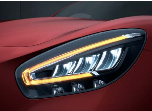
LED High Performance headlamps with Adaptive Highbeam Assist
