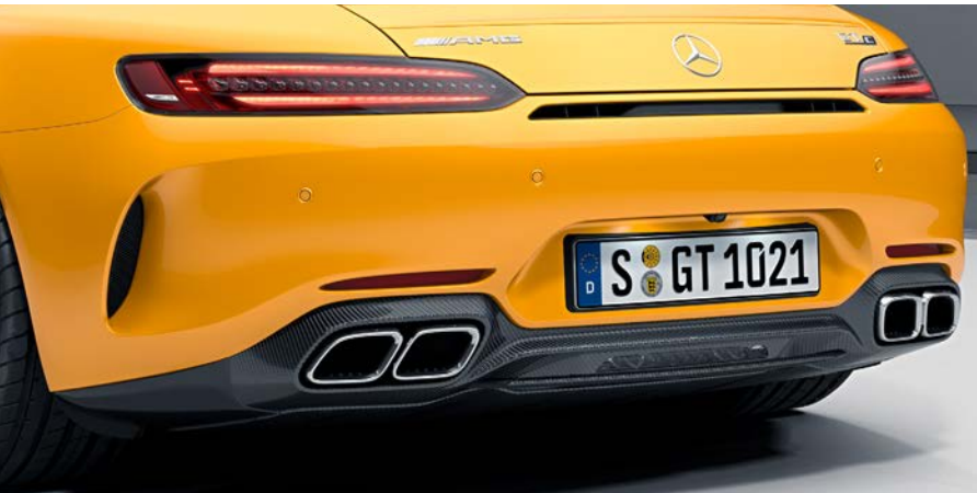
Diffuser in rear apron in carbon fibre
