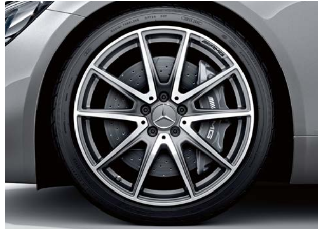
657 19"/20" AMG alloy wheels (4) – 10-spoke design, painted titanium grey front 265/35 R 19 tyres; rear 295/30 R 20 tyres
