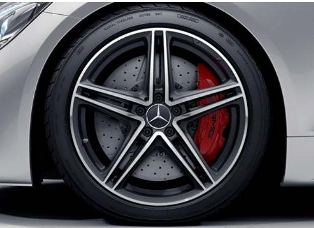
RXP 19"/20" AMG alloy wheels (4) – 5-spoke design, painted matt black front 265/35 R19 tyres; rear 305/30 R20 tyres
